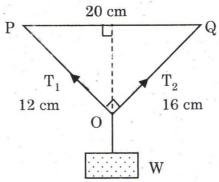
$$\frac{T_1}{OQ} = \frac{W}{PQ} = \frac{T_2}{OP} \Rightarrow \frac{T_1}{16} = \frac{W}{20} = \frac{T_2}{12} \quad \therefore \quad T_1 = \frac{4}{5} \text{ W and } T_2 = \frac{3}{5} \text{ W}$$
